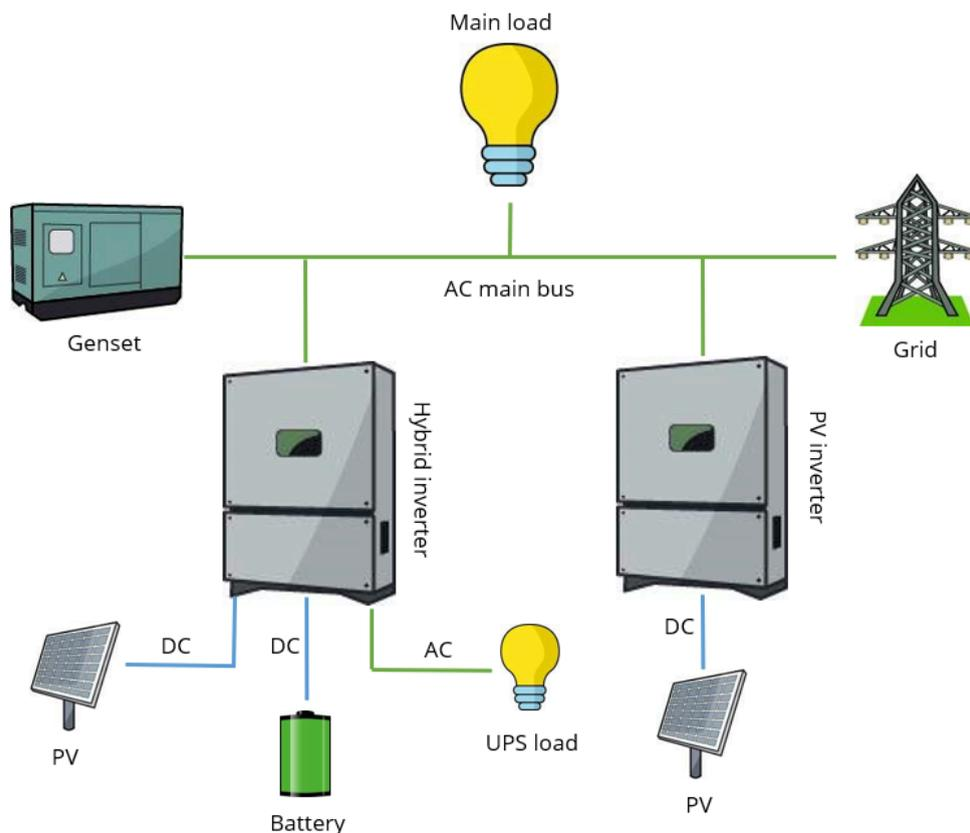
The AC production of the inverters are controlled seamlessly via a communication interface to the inverters. This interface can be either via Modbus RTU running on serial RS485 line or via Modbus TCP running on ethernet dependent on the inverter vendor and model used.
