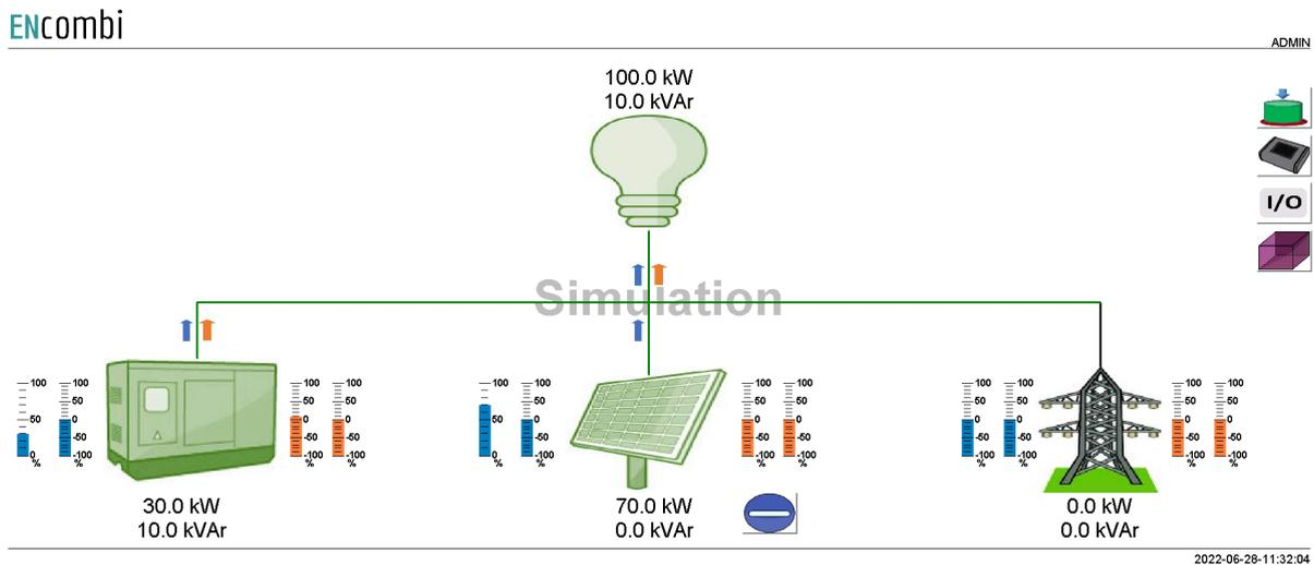
In case genset, PV or utility symbol is grayed out it means that no configuration for sensing of the associated power is made and therefore the source is interpreted as not being present by the ECpvh. The accumulated powers of the three sources as well as total consumptions are displayed.
