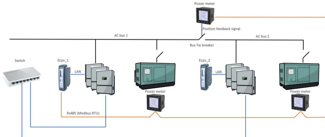
In the examples ECpvh\_1 is reading the data from the power meters via Modbus RTU. ECpvh\_2 is getting the same information but it is reading it via Modbus TCP from ECpvh\_1.
