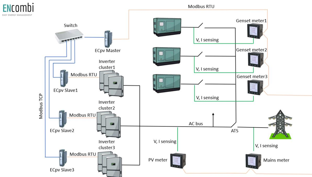
In the above example three clusters of inverters are present. These clusters can each contain up to 32 inverters and can be of another make/model than the inverters used in the other inverter clusters.
