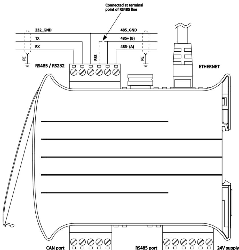
COM2 is the one found next to the power supply and COM3 is the one found next to the ethernet port.
