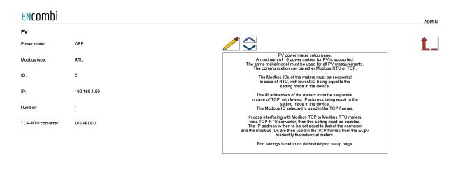
A maximum of 16 power meters for PV is supported. The same make/model must be used for all PV measurements. The communication can be either Modbus RTU or TCP. Check the link below to see which meters are supported by ECpvX. http://www.encombi.com/products/ECpvx/
