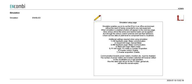
Simulation enables you to try out the ECpvX in an office environment without the need of being connected to any real equipment. When simulation is enabled, a button will appear on the monitoring overview page. Here various stimuli like active and reactive loads can be applied. Run through the various control schemes and see their behavior. Check out how data on plant level to component level is visualized.
