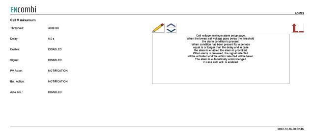
When the lowest cell voltage goes below the threshold, the alarm conditions are present. When the condition has been present for a period equal to or longer than the delay and in case the alarm is enabled, the alarm is provoked. When the alarm is provoked, the signal selected will be activated and the action selected will be taken. The alarm is automatically acknowledged in case auto ack. is enabled.
