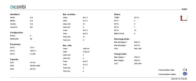
In the lower right corner communication status for the BMS is shown. In case the BMS is failing to communicate for whatever reason, communication to that specific inverter can be disabled and enabled again at a later stage on the start/stop button.
