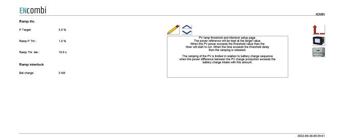
As long as the threshold delay is not elapsed, then the ECpvX will use the threshold power target as the active power reference with a unity power factor for the PV plant. The threshold timer will start to run when the PV power production exceeds the Power threshold. Once the timer elapses, then the ramping is released and the PV reference will be ramped to the actual target references.
