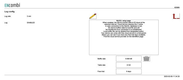
The option of using the ENcombi database requires the dedicated SW-extra "C" or time left of any complimentary free "C" trial period. The front-end for data visualization provided by ENcombi is called ECcloud. After the ECpvX has started pushing data to the ENcombi database the customer/installer can register it in ECcloud where data will be visualized immediately.
