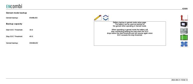
When the battery is operating in genset mode it is possible to let the battery back up if the genset fails. If the genset is failed the battery will continue operating without the genset, if genset backup is enabled.
