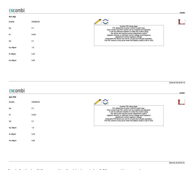
By default the PID control is disabled and the PCS control is open loop.
