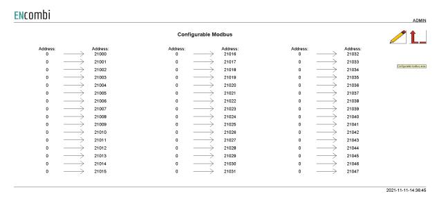
Here it is possible to tailor your own modbus mapping. Data elements that are scattered around the standard modbus map (function code 0x04) can be mapped and concentrated to the Configurable Modbus area.
