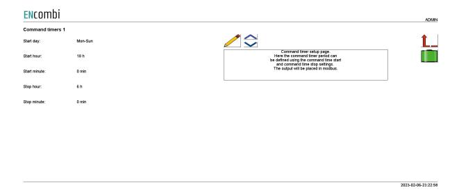
It is possible to set up 4 command timers. Type in the start day and time and stop time for the command timer. The output will be available on modbus and can be used for EClogic status/commands.
