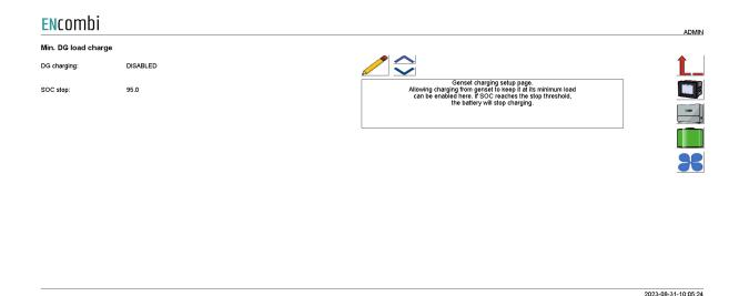
When the battery is parallel with the genset and the load is below the minimum DG load. The battery is able to charge if the SOC is below SOC stop. The battery will start charging and keep the genset at minimum DG load. When the load increases above the minimum DG load the battery will stop charging. If the SOC goes above SOC stop, the battery will stop charging as well.
