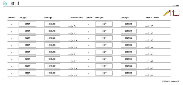
From here it is possible to set up which data should be linked to each output of the AIO module. All 16 outputs are present and it is possible to select which data to be sent out on each channel.
