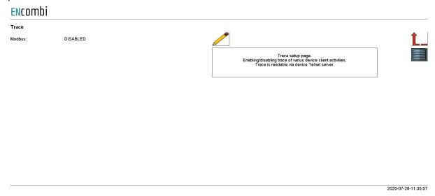
Trace is available via the built-in Telnet server. Clicking on the Telnet server button on the right hand side leads to the Telnet server setup.
