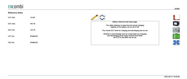
When the battery is charging it is possible to set a safety distance in order to keep the reference close to the actual charging.
