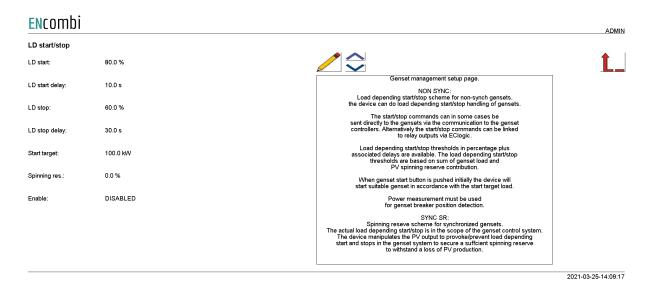
The ECpvX can do load depending start- and stop handling of gensets for two types of genset systems.
