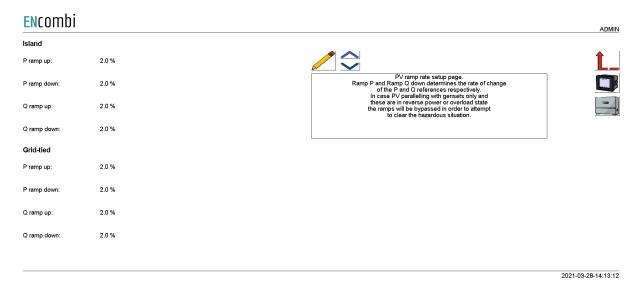
Ramp P and Ramp Q down determine the rate of change of the P and Q references respectively. Unique ramp rates are available for Island and Grid-tied operation respectively. In case PV parallelling with gensets only and these are in reverse power or
