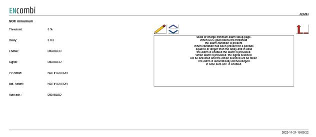
When SOC goes below the threshold, the alarm conditions are present. When the condition has been present for a period equal to or longer than the delay and in case the alarm is enabled, the alarm is provoked. When the alarm is provoked, the signal selected will be activated and the action selected will be taken. The alarm is automatically acknowledged in case auto ack. is enabled.
