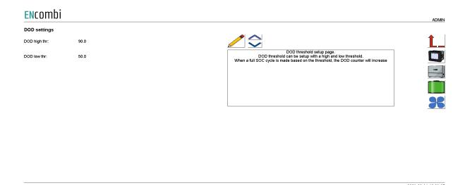
DOD threshold can be set up in order to count a DOD cycle. When a full cycle is made based on the threshold, the DOD counter will increase.
