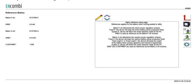
Mains P ctrl determines the active power regulation scheme.
