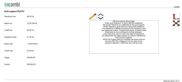
When the grid frequency is within the defined deadband, the power reference is unaffected by the grid support. When the frequency goes above or below the deadband, the power reference is then altered according to the frequency and the respective slopes. Frequencies above or below cutoff thresholds do not contribute to further alteration. Once frequency returns within the defined deadband, the references are again passed by without interference from the frequency support.
