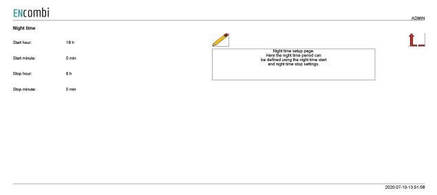
Whether the nighttime or daytime period is active, it can be used for switching the P/Q priority of the PV plant for instance.
