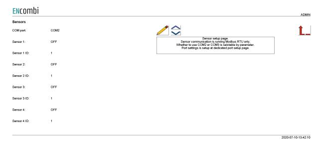
Sensor communication runs on Modbus RTU only. Whether to use sensors on COM2 or COM3 is selectable by parameter. A maximum of 4 Modbus RTU sensors can be connected to the ECpvX.
