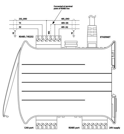
COM2 is the one found next to the power supply and COM3 is the one found next to the ethernet port.
