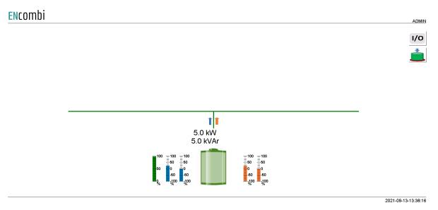
In case the battery symbol is neither gray nor green it means that the start signal is not present. In case the battery symbol is green it means that the start signal is present.
