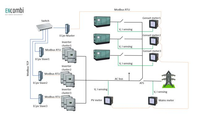
In the above example three clusters of inverters are present. These clusters can each contain up to 32 inverters and can be of another make/model than the inverters used in the other inverter clusters.
