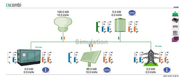
If the genset, PV, battery or utility symbol is grayed out, it means that no configuration for sensing of the associated power is made and therefore the source is interpreted as not being present by the ECpvX. The accumulated powers of the three sources as well as total consumptions are displayed.
