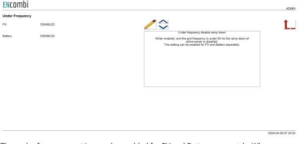
The under frequency setting can be enabled for PV and Battery separately. When enabled, the active power is prohibited from ramping down while the frequency is under 50 Hz.
