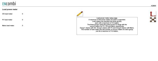
Above page there are 3 options to select load power meters. If the DG load meter is selected, the power meter protocol is selected on the DG power meter page. The ID of the load meter will be the next ID after the DG power meter.
