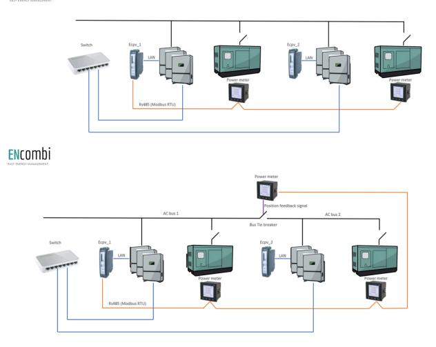
In the examples ECpv\_1 is reading the data from the power meters via Modbus RTU. ECpv\_2 is getting the same information but it is reading it via Modbus TCP from ECpv\_1.
