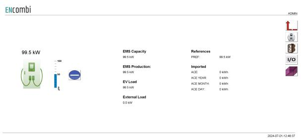
The current charging capacity, power production, EV charger power consumption, and the external load are shown in the left column. The right column shows the total power limit target and reference for the charging stations. The accumulated energy consumption is also shown here.
