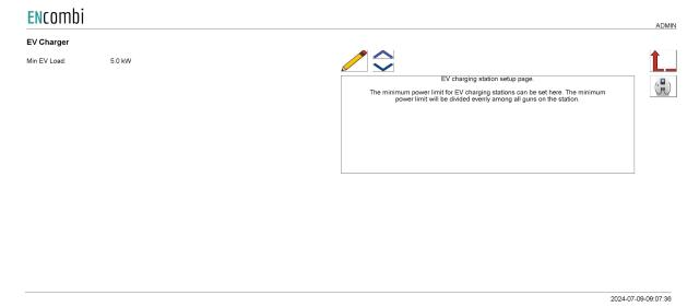
The minimum power limit is distributed evenly between all guns on the station based on the Guns per station setting.
