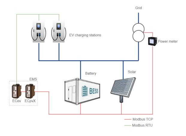
EVCev will communicate with the EV charging stations and the EMS via Modbus. Based on the available generating capacity reported by the EMS, the power limit for each EV charging station is set. The ECpvX acts as EMS which monitors and controls the Battery, PV inverters, and grid connection. The EMS decides what the generating capacity of the plant is, based mainly on the size of the grid connection and SOC of the Battery. Consult the ECpvX User Manual for more information on the ECpvX.
