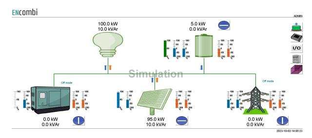
If the genset, PV, battery or utility symbol is grayed out, it means that no configuration for sensing of the associated power is made and therefore the source is interpreted as not being present by the ECpvX. The accumulated powers of the three sources as well as total consumptions are displayed.
