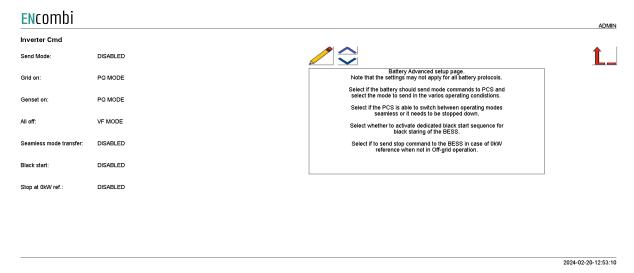
For some protocols it is possible to select whether the ECpvX should send mode commands to the PCS. Then the ECpvX will send the mode based on the operating condition. The operating mode for the various operating conditions can be set. All operating modes may not be supported by a given PCS. The support modes for the ECpvX to send is:
