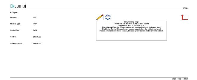
A maximum of 1 ECsync cabinet is supported by a single ECpvX. The ECpvX can interface to the ECsync cabinet via Modbus RTU or Modbus TCP. The data read from the ECsync cabinet will be visualized on a dedicated page. Enable the Control if to use the dry contact outputs from the cabinet and send manual commands like mode change, breaker open/close etc. to the ECsync cabinet. The relay control is set up via EClogic whereas the various commands are set from the ECsync monitoring page.
