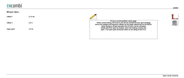
When synchronizing, the ECpvX will use the sensed ECsync grid readings minus the voltage and frequency offsets as the target references for the BESS. When going to off grid operation the ECsync will be unloaded initially and first open its breaker when the loading is below the open threshold point. The open point threshold refers to the rating of the PCS.
