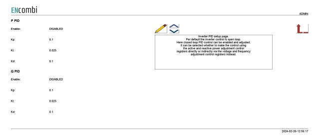
By default the PID control is disabled and the Inverter control is open loop. Closed loop control can help achieve the desired power output when controlling multiple PV inverters even if one or more of them do not produce the desired output. Active and Reactive power PID control can be enabled separately.
