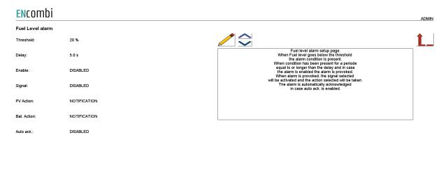
When fuel level goes below the threshold, the alarm conditions are present. When the condition has been present for a period equal to or longer than the delay and in case the alarm is enabled, the alarm is provoked. When the alarm is provoked, the signal selected will be activated and the action selected will be taken. The alarm is automatically acknowledged in case auto ack. is enabled.
