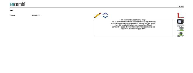
The ECpvX can take in various commands including power and reactive power commands for both PV and BESS via ECapi. This enables an online optimizer service provider to control the PV and BESS via ECapi thereby eliminating the need for installing any additional HW on site. The API setting must be enabled in order to have the ECpvX accepting commands applied via ECapi. Consult the ECapi documentation on which commands are available and how to apply them.
