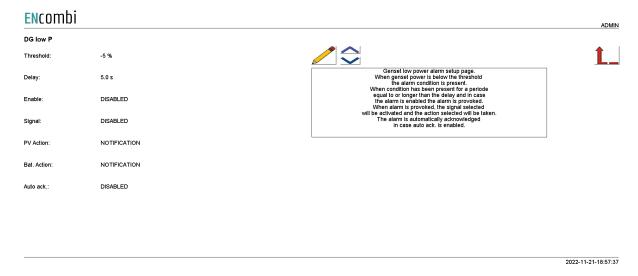
When the genset power is below the threshold, the alarm condition is present. When the condition has been present for a period equal to or longer than the delay and in case the alarm is enabled, the alarm is provoked. When the alarm is provoked, the signal selected will be activated and the action selected will be taken. The alarm is automatically acknowledged in case auto ack. is enabled.
