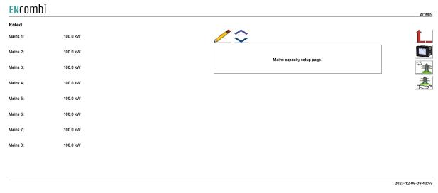
A total of 16 utility connections are supported. Above page is one of two pages available for setting up the rated mains transformer sizes.
