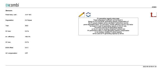
GC compensation selection determines if and how to do generating capacity compensation of the PV panels. The ECpvX uses PV panel generating capacity for handling curtailment counters and PV performance ratios. Supported methods are:
