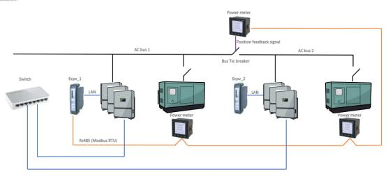
In the examples ECpv\_1 is reading the data from the power meters via Modbus RTU. ECpv\_2 is getting the same information but it is reading it via Modbus TCP from ECpv\_1.
