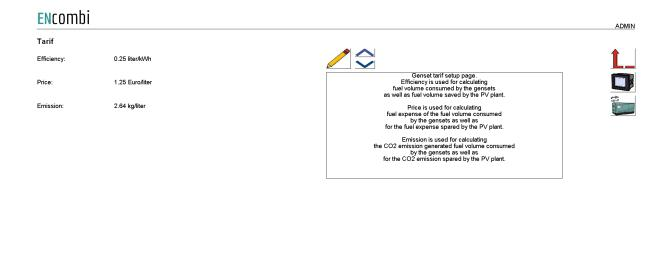
Efficiency is used for calculating fuel volume consumed by the gensets as well as fuel volume saved by the PV plant.
