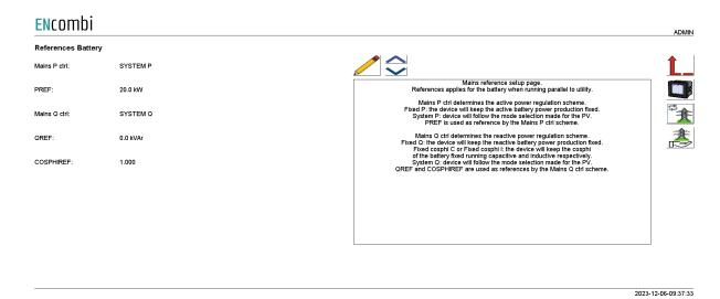
Mains P ctrl determines the active power regulation scheme.
