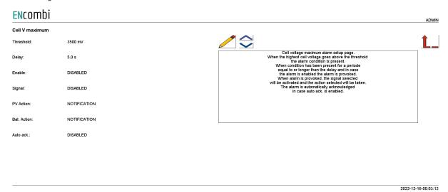
When the highest cell voltage goes above the threshold, the alarm conditions are present. When the condition has been present for a period equal to or longer than the delay and in case the alarm is enabled, the alarm is provoked. When the alarm is provoked, the signal selected will be activated and the action selected will be taken. The alarm is automatically acknowledged in case auto ack. is enabled.
