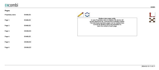
In case Proprietary slave is enabled, the ECpvX will accept instructions to be received over modbus via a dedicated proprietary modbus profile. The various instructions are furthermore grouped together in different pages that need to be enabled individually. Consult the Modbus slave documentation on ENcombi website for detailed information about the proprietary modbus profile.
