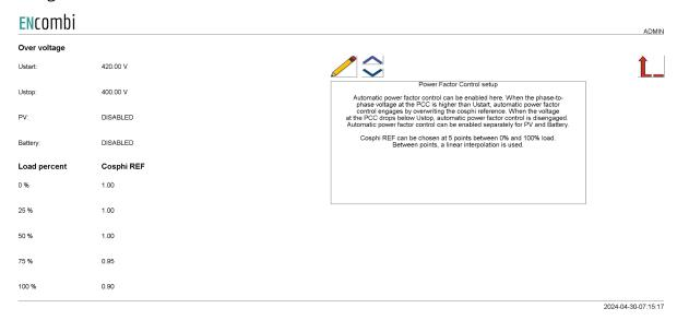
This setting starts to overwrite the cosphi reference when the grid voltage measured by the mains meter exceeds Ustart, and stops overwriting the cosphi reference once the grid voltage drops below Ustop.
