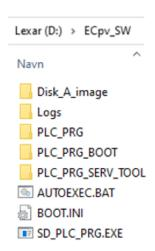
Then insert the USB stick into the ECpvX and press the binoculars button to start the SW update. When the SW update is completed successfully, then you can safely revert to the ECpvX application. If the SW is interrupted and it fails, then remain in the Boot application and try to update the SW once again. Do not return to the ECpvX application until the SW update is completed successfully.
