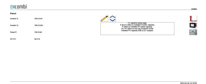
The S and Q refer to the total installed PV inverter capacity whereas the Panel P refers to the total installed PV panel capacity, that is both AC and DC coupled. The PV DC percentage refers to how big a part of the total installed Panel capacity that is DC coupled to the BESS.
