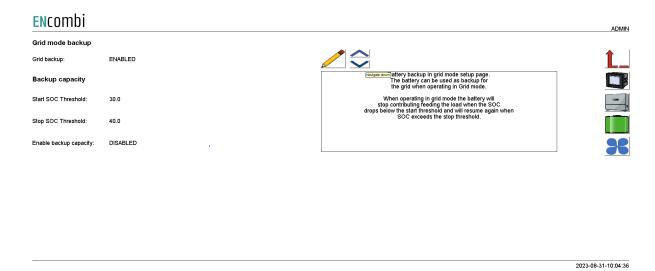
When the battery is operating in grid mode it is possible to let the battery backup if the grid fails. If the grid is failed the battery will continue operating without the grid, if grid backup is enabled.
