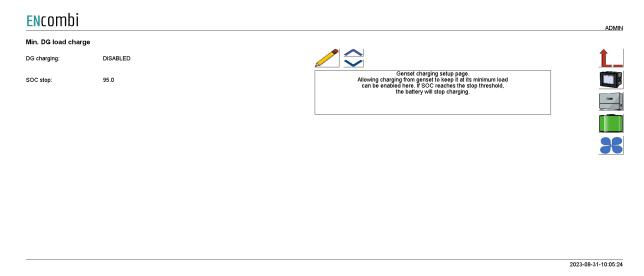
When the battery is parallel with the genset and the load is below the minimum DG load. The battery is able to charge if the SOC is below SOC stop. The battery will start charging and keep the genset at minimum DG load. When the load increases above the minimum DG load the battery will stop charging. If the SOC goes above SOC stop, the battery will stop charging as well.
