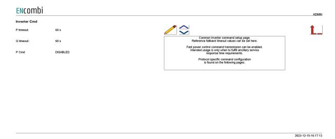
These settings are common for all inverters and may or may not apply to the specific inverter make/model selected. Fallback timeouts for reverting to a predefined production level in case of loss of communication can be set up.
