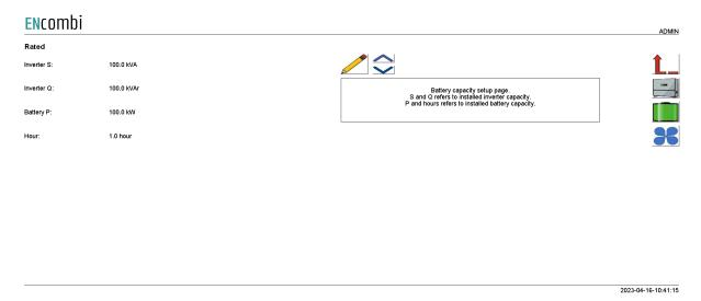
The S and Q ratings refer to the Power Conversion System whereas the P and Hour refer to the installed battery capacity.
