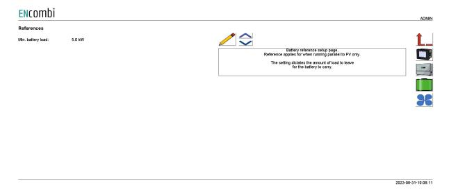
When the battery is parallel with PV only, it can be selected how much loading there should be kept on the battery. The ECpvX will seek to have the PV pick up any excessive load.
