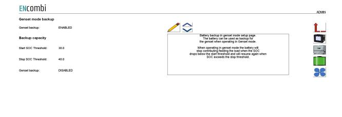
When the battery is operating in genset mode it is possible to let the battery back up if the genset fails. If the genset is failed the battery will continue operating without the genset, if genset backup is enabled.
