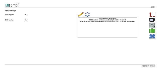
DOD threshold can be set up in order to count a DOD cycle. When a full cycle is made based on the threshold, the DOD counter will increase.
