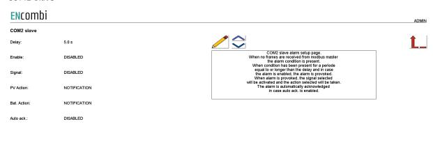
When no frames are received from the modbus RTU master, the alarm condition is present. When the condition has been present for a period equal to or longer than the delay and in case the alarm is enabled, the alarm is provoked. When the alarm is provoked, the signal selected will be activated and the action selected will be taken. The alarm is automatically acknowledged
