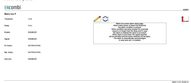
When the mains power is below the threshold the alarm condition is present. When the condition has been present for a period equal to or longer than the delay and in case the alarm is enabled, the alarm is provoked. When the alarm is provoked, the signal selected will be activated and the action selected will be taken. The alarm is automatically acknowledged in case auto ack. is enabled.
