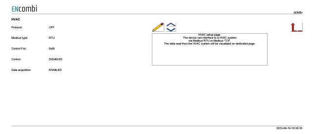
A maximum of 1 HVAC system is supported by a single ECpvX. The communication can be either Modbus RTU or TCP. On the ENcombi website you can see which HVAC systems that are supported. Should your preferred inverter not be on the list already, contact ENcombi to request the adding of it. http://www.encombi.com/products/ecpvx/
