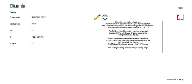
Note that the ECpvX will be reading data from multiple power meters from a single ECpv. In the above configuration the ECpvX will be reading data from two genset power meters from an ECpvX having IP address 192.168.1.79.
