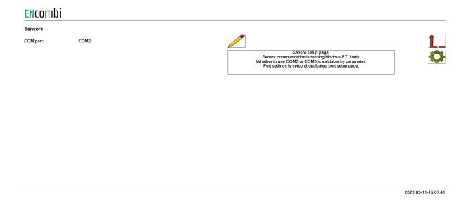
Afterwards, clicking on the setup button on the right hand side leads to the Sensor configuration itself where the Sensor modules communication settings can be adjusted and the Sensor modules can be searched and identified.
