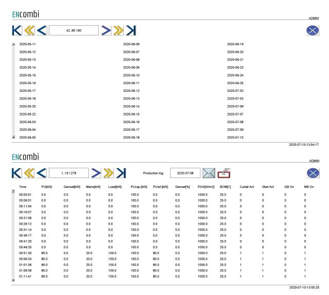
Note that the column heading of the production log shown is not actually included in the actual file being transferred by FTP. The files only contain the data itself.
