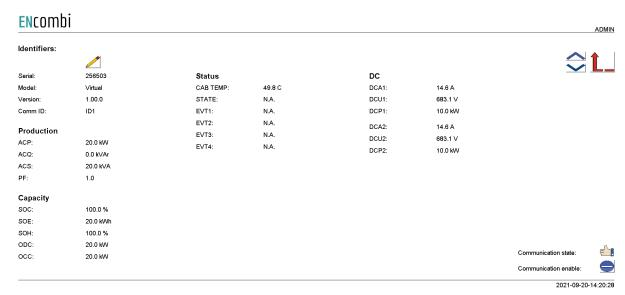
In the upper left corner the label of the inverter can be changed. In the lower right corner communication status for the specific inverter is shown. In case the inverter is failing to communicate for whatever reason, communication to that specific inverter can be disabled and enabled again at a later stage on the start/stop button. In the upper right corner it is possible to toggle between the pages.
