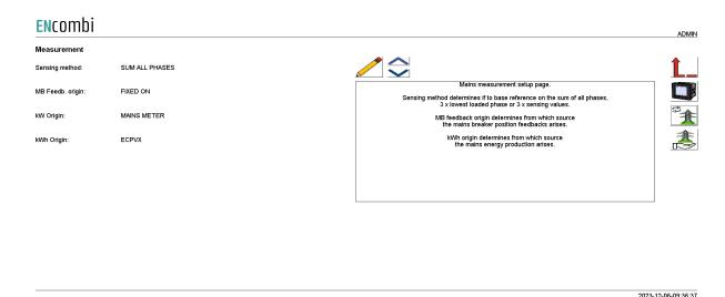
Sensing method determines what power readings to base the calculated references upon. Three options are available.
