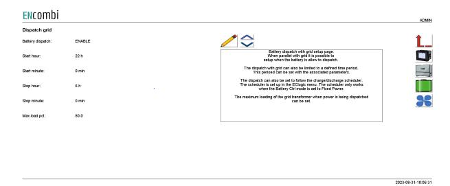
When the battery is parallel with the grid it is possible to select if the battery should be able to dispatch power. It is possible to select if the battery should be able to dispatch all the time or only in a defined period of time. The maximum loading of the transformer allowed can be adjusted by the dedicated setting. If dispatch is disabled, the battery will still help the grid if the load is bigger than the grid capacity.
