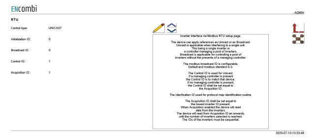
The ECpvX can apply references as Unicast or as Broadcast. Unicast is applicable when interfacing to a single unit. This being a single inverter or a controller managing a pool of inverters. Broadcast is applicable for controlling a pool of inverters without the presence of a managing controller.
