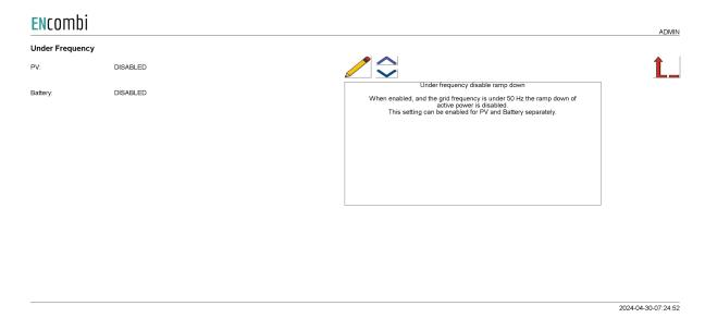
The under frequency setting can be enabled for PV and Battery separately. When enabled, the active power is prohibited from ramping down while the frequency is under 50 Hz.
