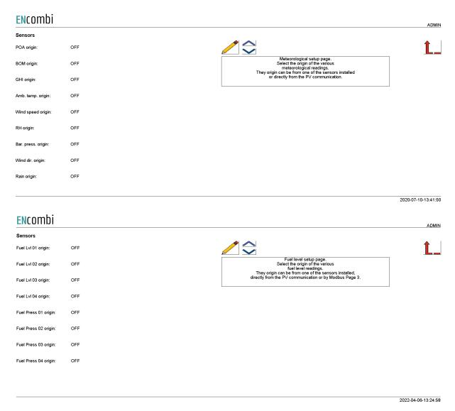
Above page holds the list of all meteorological readings supported. The origin of these readings can be selected as either Modbus RTU based sensors, inverter communication, Modbus page 3 or by EClogic.
