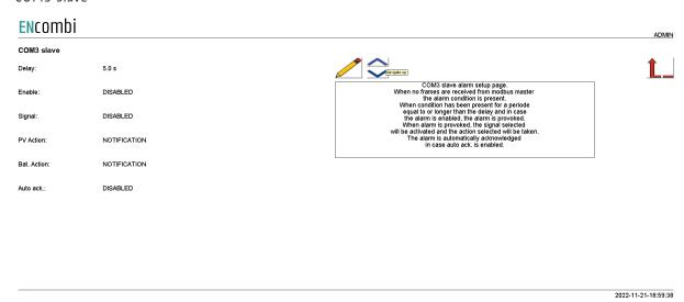
When no frames are received from the modbus RTU master, the alarm condition is present. When the condition has been present for a period equal to or longer than the delay and in case the alarm is enabled, the alarm is provoked. When the alarm is provoked, the signal selected will be activated and the action selected will be taken. The alarm is automatically acknowledged in case auto ack. is enabled.
