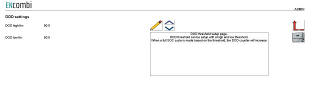
DOD threshold can be set up in order to count a DOD cycle. When a full cycle is made based on the threshold, the DOD counter will increase.
