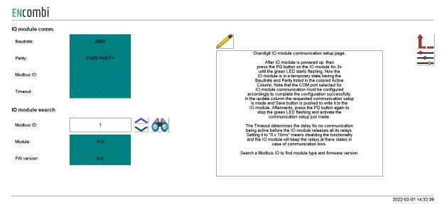
It is possible to set up the Overdigit IO module with the tool.
