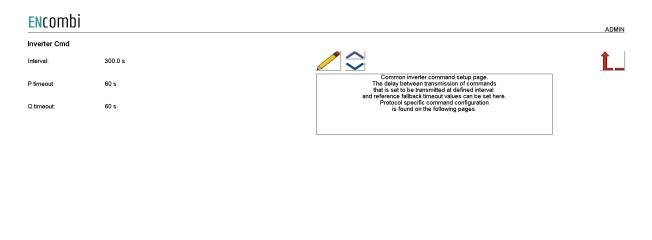
These settings are common for all inverters and may or may not apply to the specific inverter make/model selected. Here the delay between transmission of commands that is set to be transmitted at a defined interval can be set. Furthermore the fallback timeouts for reverting to a predefined production level in case of loss of communication can be set up.
