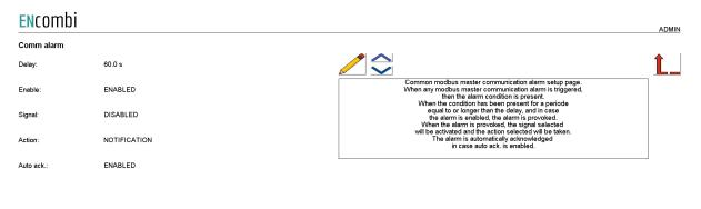
This alarm condition is present in case any of the modbus master communication alarms for the inverter, power meter, sensor or IO communication are raised. When the condition has been present for a period equal to or longer than the delay and in case the alarm is enabled, the alarm is provoked. When the alarm is provoked, the signal selected will be activated and the action selected will be taken. The alarm is automatically acknowledged in case auto ack. is enabled.
